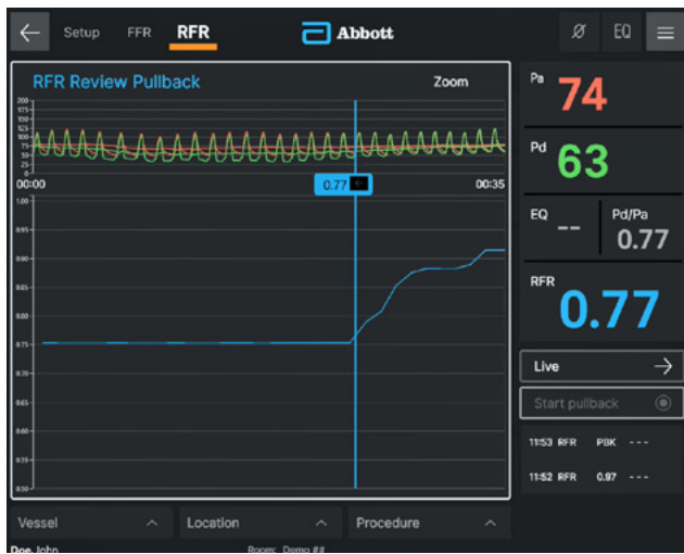
2a. Physiology Review screen displaying pressure gradient and RFR value
