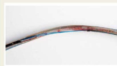
Figure 2 Extracted Riata lead demonstrating that the conductors are outside the lead body.
