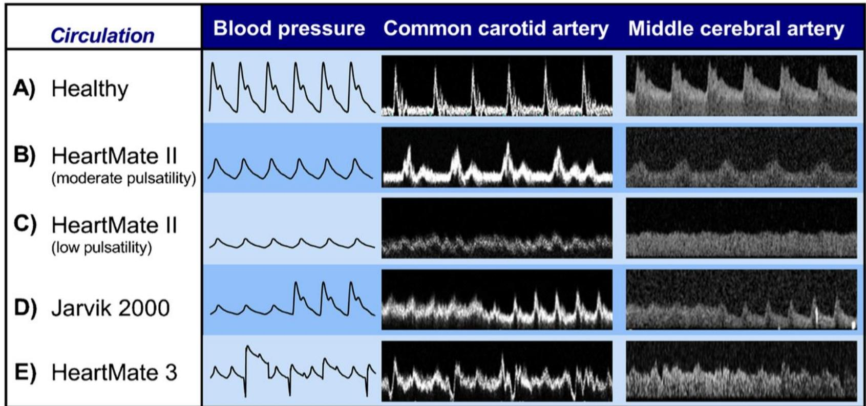
HeartMate II, Jarvik 2000: axial flow pump [MAP target  $\leq 90$  (85) mmHg];
